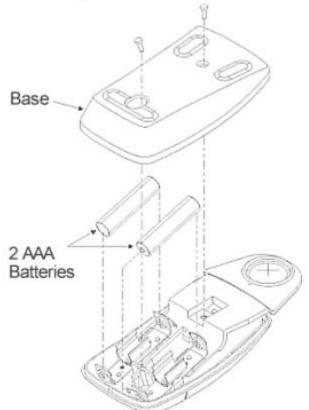
**NOTE:** When you replace the cordless cursor batteries, the cursor will reset to the default frequency. If you changed the frequency of the cursor before replacing the batteries, you will need to do so again after replacing the batteries (see the *Reducing Monitor Interference* section in *Troubleshooting*).
