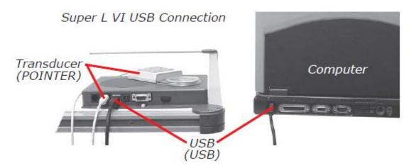
**NOTE:** Power is supplied through the USB port. No additional power source is needed for this installation.
