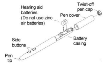
**NOTE:** When you replace the pen batteries, the pen will reset to the default frequency. If you changed the frequency of the pen before replacing the batteries, you will need to do so again after replacing the batteries (see the *Reducing Monitor Interference* section in *Troubleshooting*).
