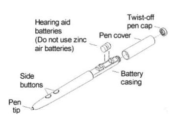
**NOTE:** When you replace the pen batteries, the pen will reset to the default frequency. If you changed the frequency of the pen before replacing the batteries, you will need to do so again after replacing the batteries (see the *Reducing Monitor Interference* section in *Solving Problems*).
