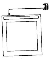
3. Connect the 25-pin D connector of the interface cable into the host communications port.
