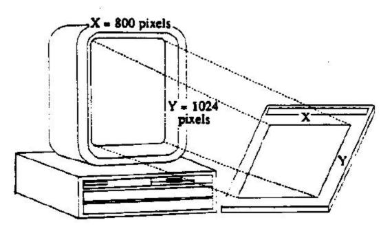
In this case, ensure the length of the corresponding tablet axis divides evenly into the other device's resolution. If it does not, the tablet truncates the resolution value to a whole number.
