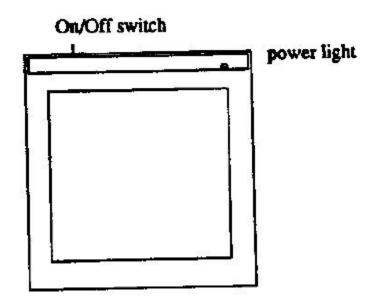
The power light is lit when the tablet is on. It's also a proximity indicator that remains lit when the stylus/cursor is in-prox. It blinks when the stylus/cursor is out-of-prox. If the light blinks when the stylus/cursor is in-prox, then the tablet is malfunctioning. Turn it off for 10 or 20 seconds, and then turn it on again. If it fails again, have it serviced.
