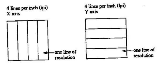
The higher the resolution, e.g. 100 lpi or 200 lpi, the narrower the bands of resolution become. Eventually, the bands become so narrow that they are easier to conceptualize as *lines* of no measurable width.
