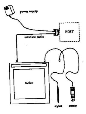
The tablet is similar to a drawing board. The stylus and cursor are handheld devices that are used for pointing or drawing on the tablet. The interface cable connects the graphics tablet to the host (computer).
