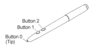
*Click Tip Pen:* Primarily used for tracing and menu picking. To use the pen, press down until you feel the tip click.
