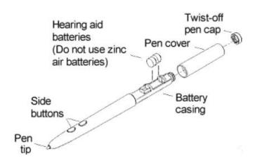
**NOTE:** When you replace the pen batteries, the pen will reset to the default frequency. If you changed the frequency of the pen before replacing the batteries, you will need to do so again after replacing the batteries (see the *Reducing Monitor Interference* section in *Troubleshooting*).
